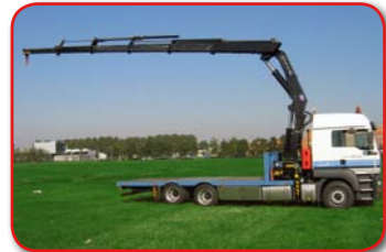
The sophisticated dual link arm system on the HMF 4220 Series ensures a uniform speed and lifting capacity in the entire working area.
