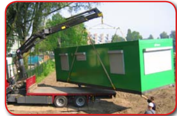
The picture gives you an impression of the powerful load moment close to the column. The maximum lifting capacity of an HMF 4220-K2 is 13.5 tonnes.
